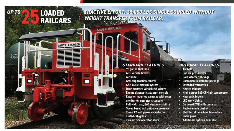
The Commander Series Shuttlewagon shares many of the same features as the larger Navigator but comes in a smaller package. It is designed to complete up to 35,000 lbs of tractive effort from one coupler. Compact yet powerful, the Commander Series pulls as much weight as other manufacturers' largest models.
