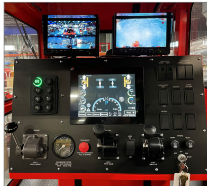
180-degree rotating console with multifunction display. Dual four-way air suspension seats for operation from either side of cab in rail mode. Shown with 4-camera surround.
