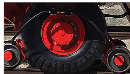
Patented rail guidance system: two independent drive wheel trucks supported on rotating bearing with eight 16" AAR profile guide wheels. ABS & traction assist provide more control while reducing maintenance costs.
